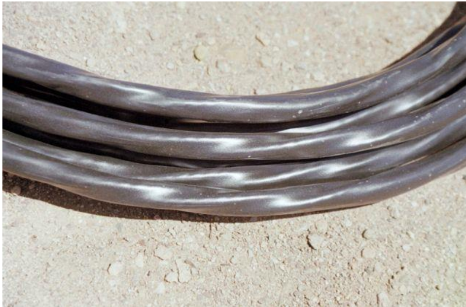
Three-conductor ROMEX, which happens to be twisted inside the sleeve. The twisting can be seen through the outer sleeve.
