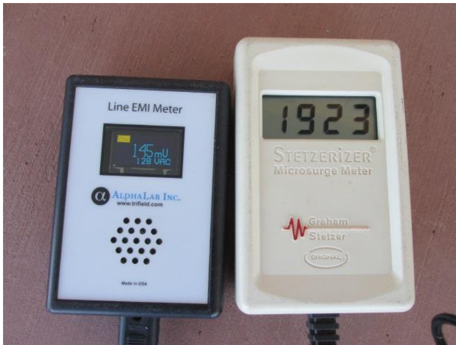
Two meters show very high levels of dirty electricity from a high-quality name-brand inverter. (Measured with inverter only, to avoid other possible sources of dirty electricity.)
