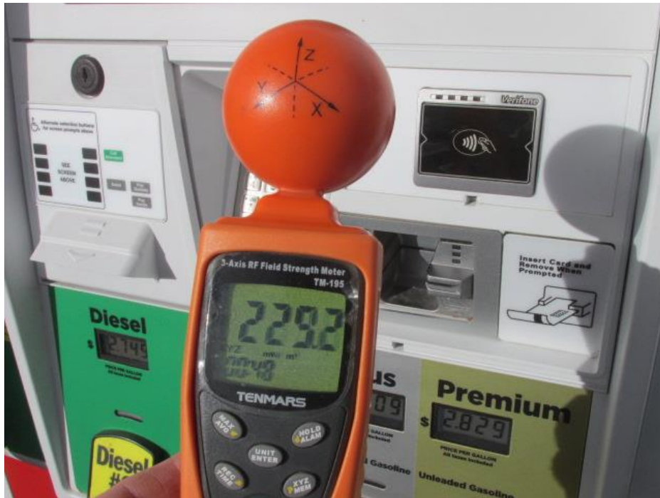
Demonstrating wireless radiation from a gas pump's NFC payment system, even when it is not in use. It measures 229,200 uW/m 2 .
