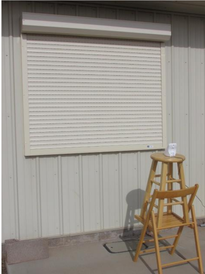
Transmitter located outside with the RF meter inside. Shutters closed.
