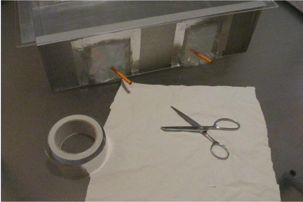
Cutting the cotton bedsheet to use as gasket.
