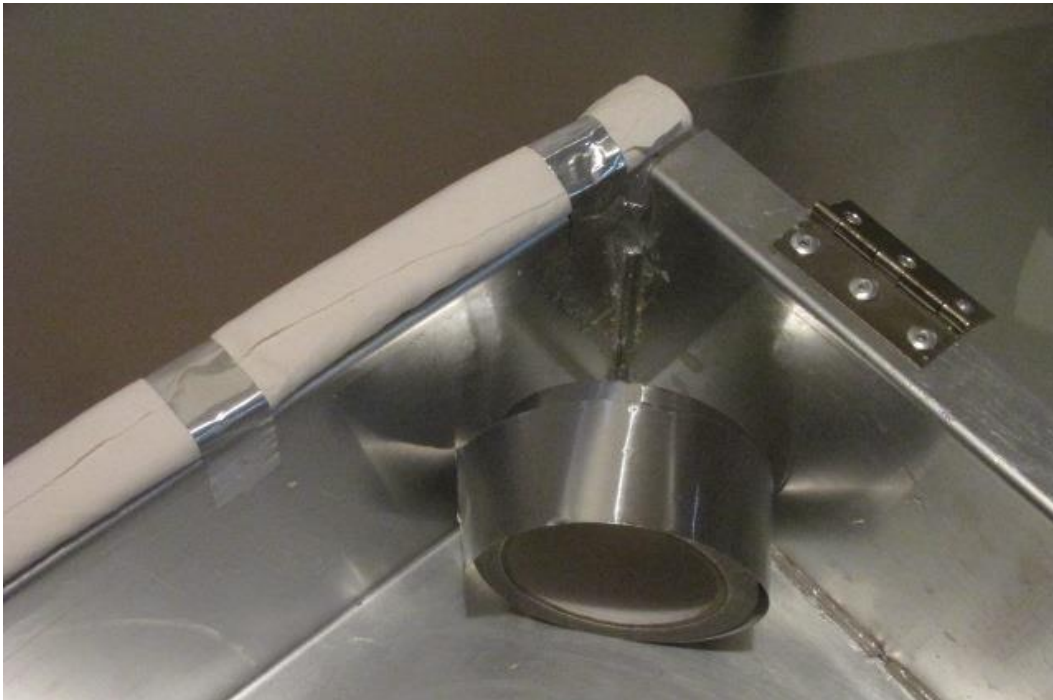
Installing the gasket.
