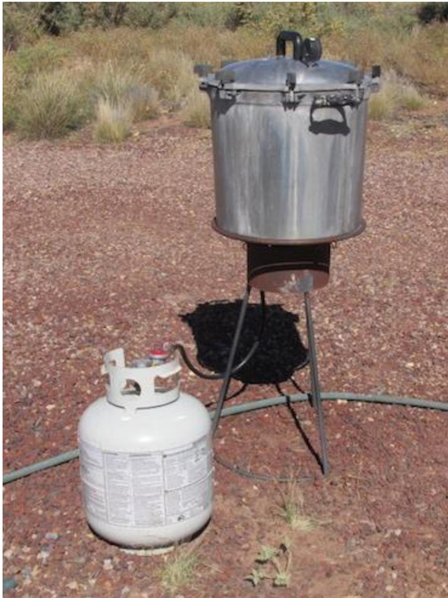
*A large pressure cooker used to detox clothes. It needs a hefty propane burner to get hot.*
