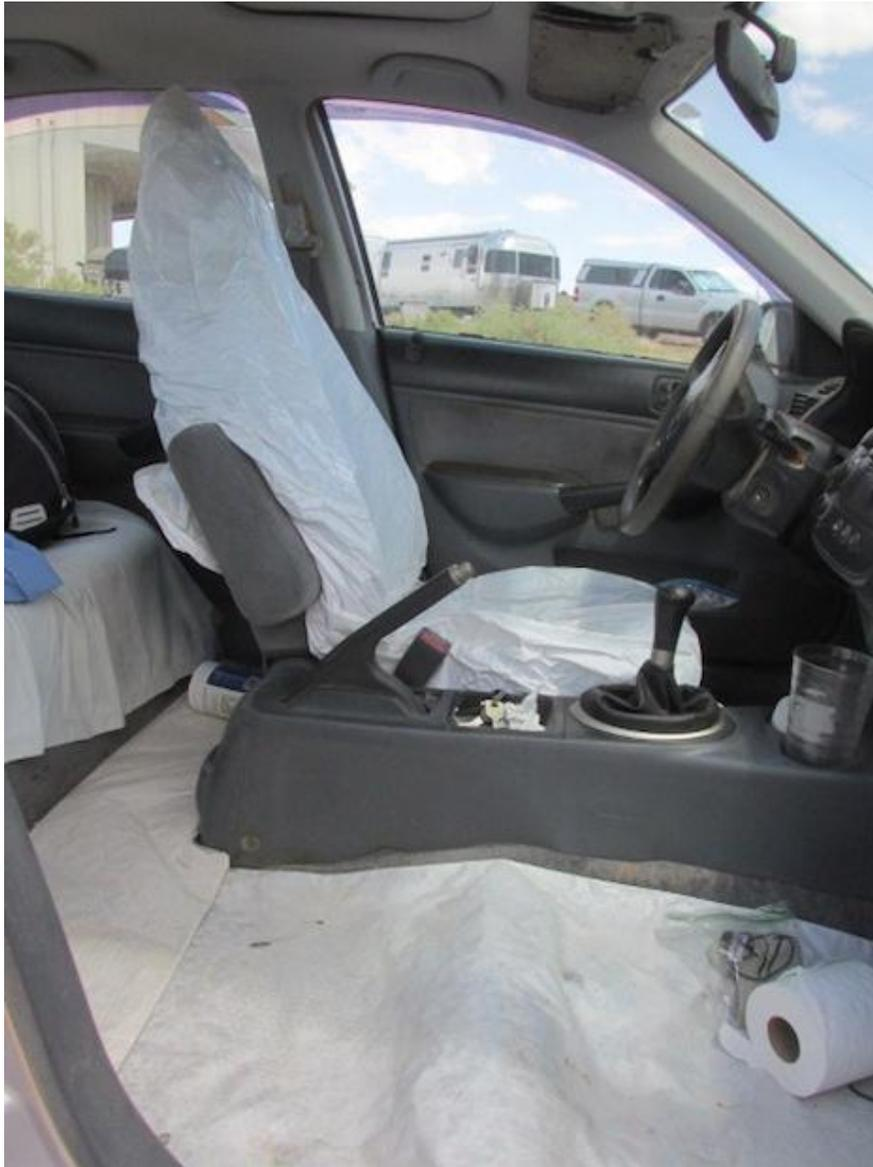
*Seat and floor covered with polyethylene plastic. One seat is also removed.
