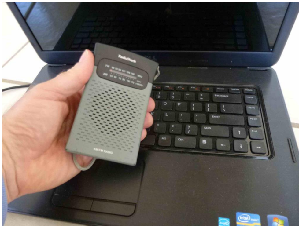
Instruments to measure EMF are helpful. Here, a simple AM radio demonstrates radiation from a laptop computer with no wireless transmitters.
