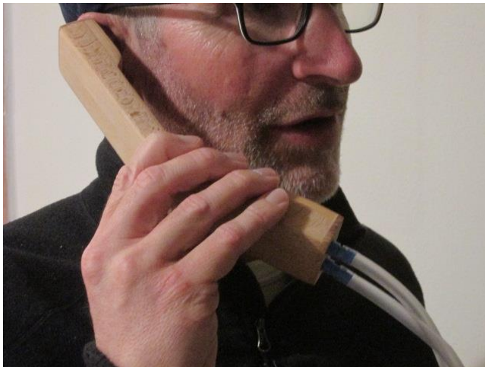
Non-electric tube phone. The sound travels in tubes to/from a box with speaker and microphone.
